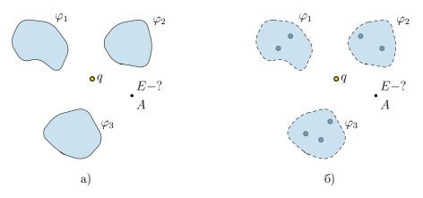
Pис. 1: The figure on the left is the original problem, and the figure on the right is an equivalent problem, with image charges instead of conductors.
